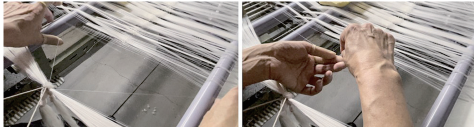
Figure 17. Hand tying-in (연구자 촬영 2021).
